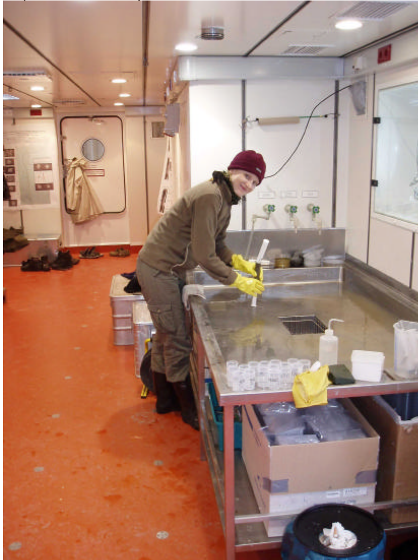
Fig. 8: Slicing a syringe subsample in the ship's deck laboratory
