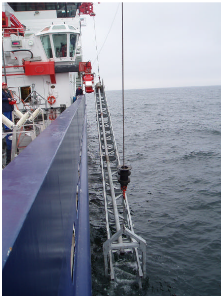
Fig. 3: Gravity-corer with 18 m long steel tube was used in Arkona Basin.
