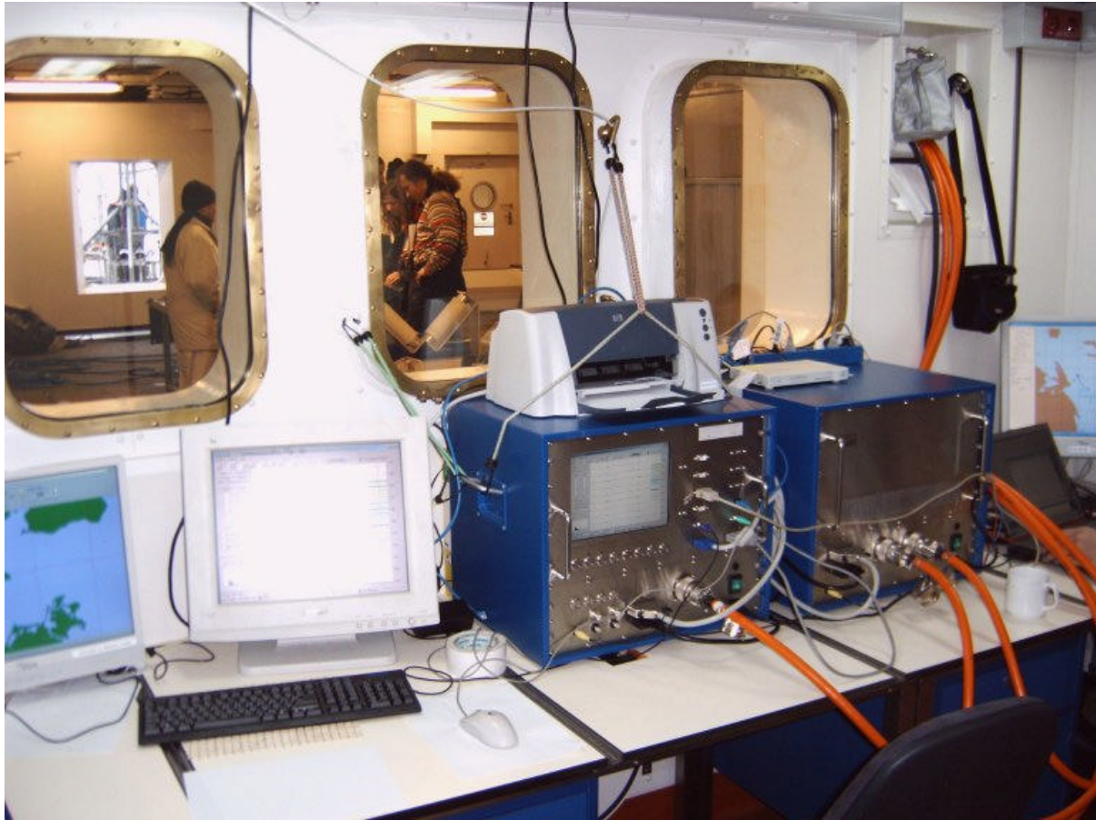
Fig. 1: The portable parametric sediment echosounder SES2000deep, recording and transmitting units (blue boxes).
