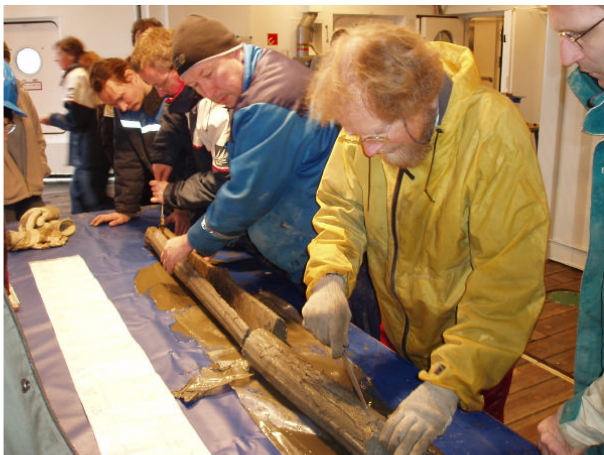
Fig. 5: Core opening in the laboratory.
